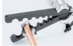
Insert a tube until it hits TA504FG.
