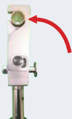
Position tubing in groove and engage with hook.
