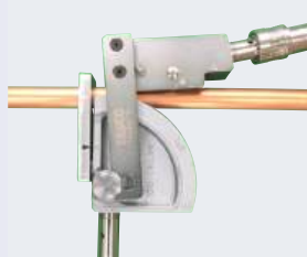
Set lever guide handle on wheel handle.
